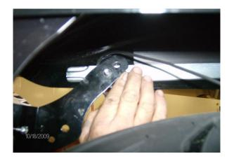
AFTER ASSEMBLY OF LICENSE PLATE AND LIGHT TO THE NEW FRAME, INSTALL THE NEW FRAME TO THE MOTORCYCLE. THE SPACER WASHER GOES BETWEEN THE NEW FRAME AND THE MOTORCYCLE AT THE FRONT HOLE
