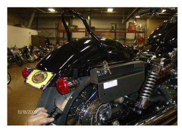
INSTALL TURN SIGNALS TO NEW FRAME POSITION NEW FRAME UNDER FENDER, LEVEL TURN SIGNALS AND TIGHTEN ALL BOLTS. ROUTE ALL WIRING TO AVOID CONTACT WITH TIRE. REINSTALL SHOCKS
